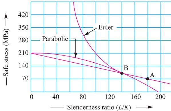
Fig. 16.4. Relation between slenderness ratio and safe stress.
