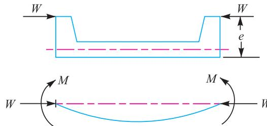
Fig. 16.5. Long column subjected to eccentric loading.
