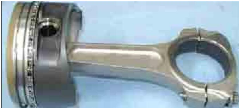
Piston rod is made of mild steel.
