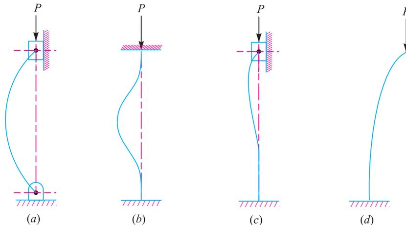
Fig. 16.1. Types of end conditions of columns.
